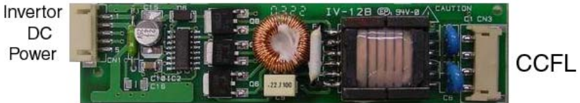
Figure 3.8: Locating Connectors on DC/AC Inverter
