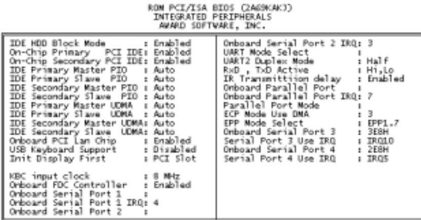
**Figure 9-8: Integrated peripherals screen**
