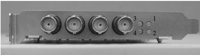
Figure 1.4 LED indicator location
