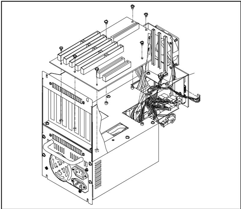
**Figure 3-1: Removing the passive backplane**
