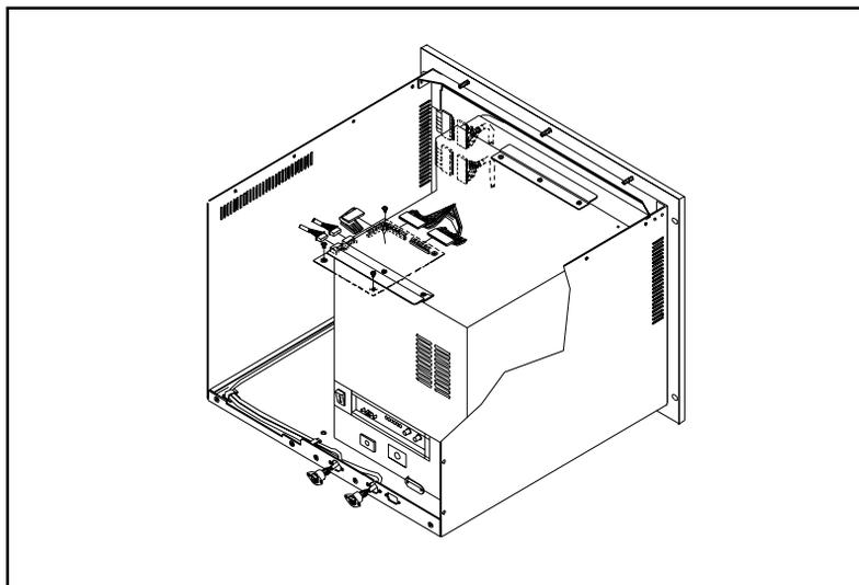
**Figure 3-7: Removing the keyboard translator**
