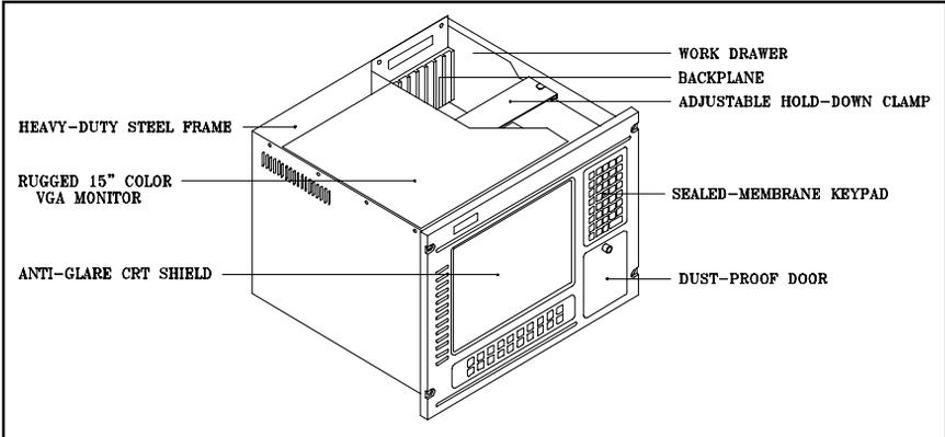
Figure 1-2: Front panel layout
