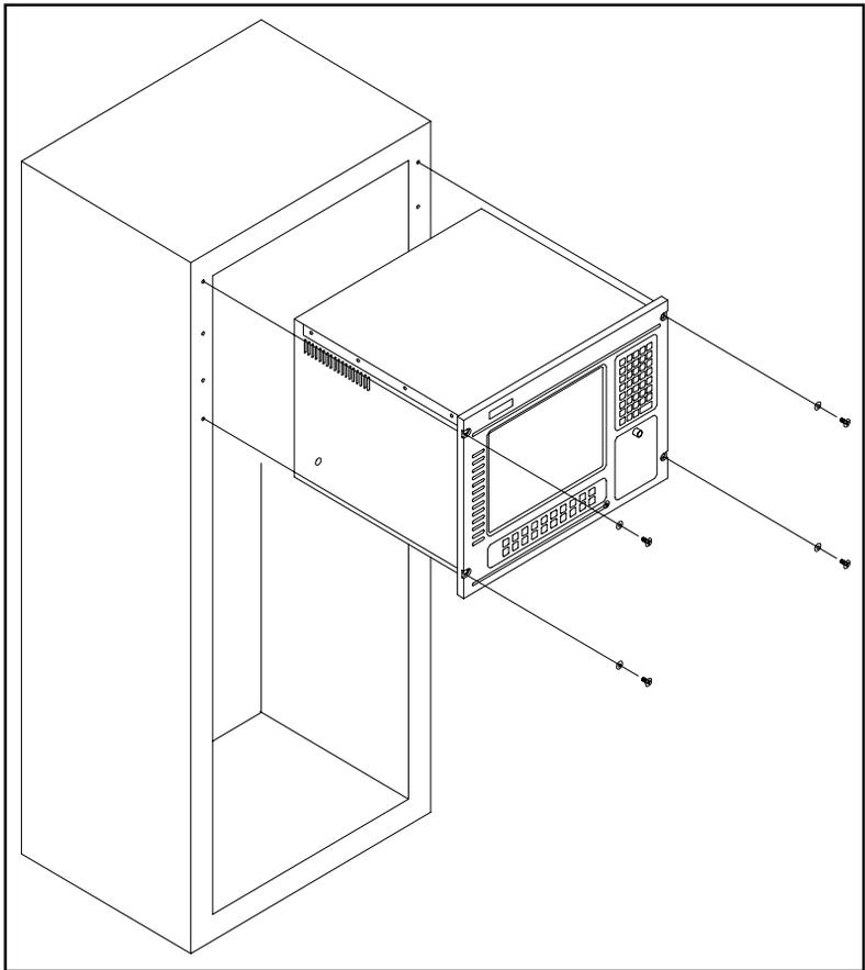
**Figure 2-5: Rack mounting the AWS-825B/PB**
