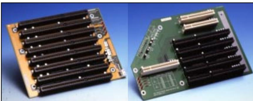
**Figure 1-1: The PCA-6108C and PCA-6107P2 passive backplanes**
