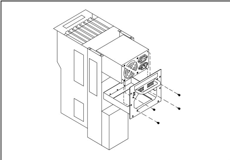
**Figure 3-2: Removing the power supply**
