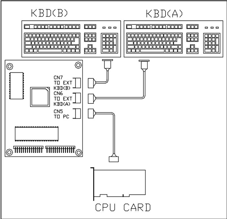
**Figure 3-6: Keyboard translator input/output (schematic)**
