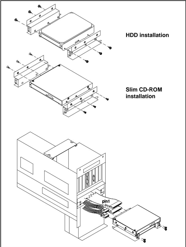
**Figure 2-3: Installing optional drives**
