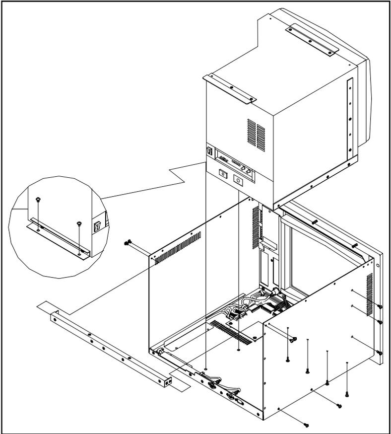
**Figure 3-4: Removing the CRT monitor - final steps**
