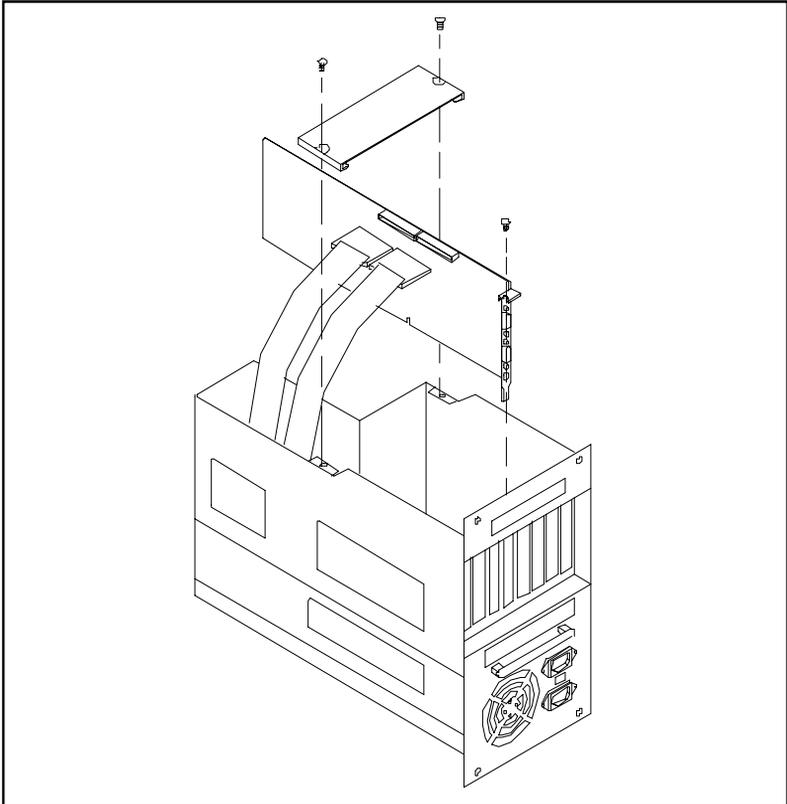
**Figure 2-2: Installing add-on cards**
