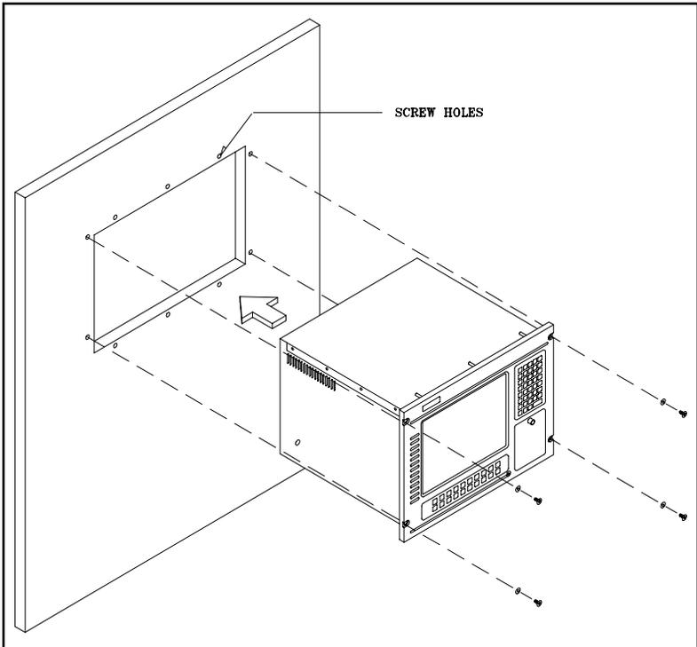
**Figure 2-6: Panel mounting the AWS-825B/PB**
