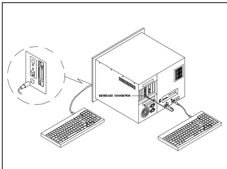
**Figure 3-5: Keyboard translator input/output (actual)**
