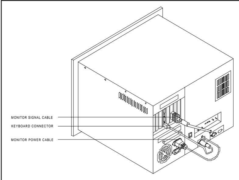
**Figure 2-4: Cables on the rear panel**
