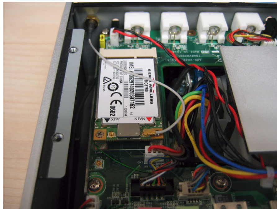
Figure 2.30 Connect the SMA Cable to the miniPCIe card module
