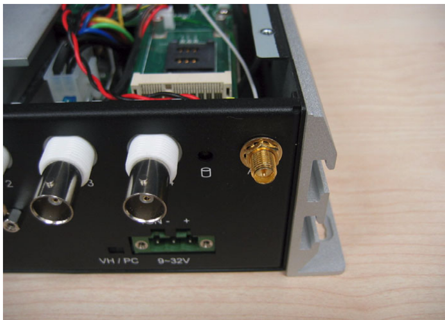
Figure 2.27 Knock out ANT hole and screw the SMA Cable into the front panel
