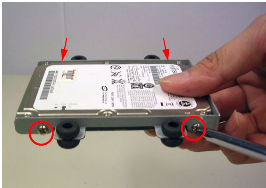
Figure 2.18 Assemble HDD and HDD frame with 4 screws
