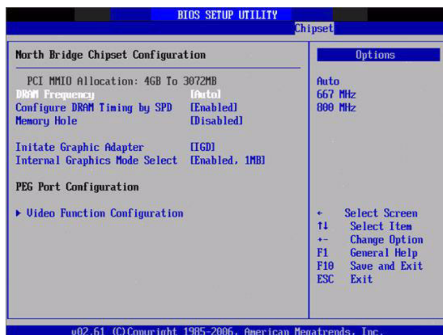
Figure 3.24 North Bridge Configuration
