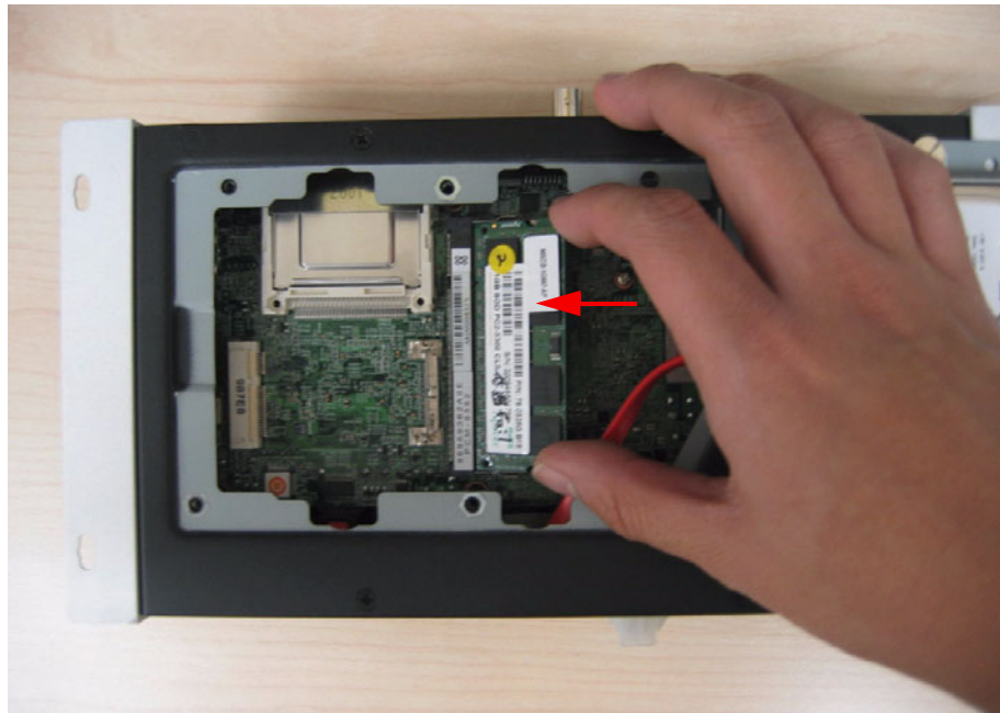
Figure 2.21 Install the memory module into the SO-DIMM socket at the bottom of the Main board
