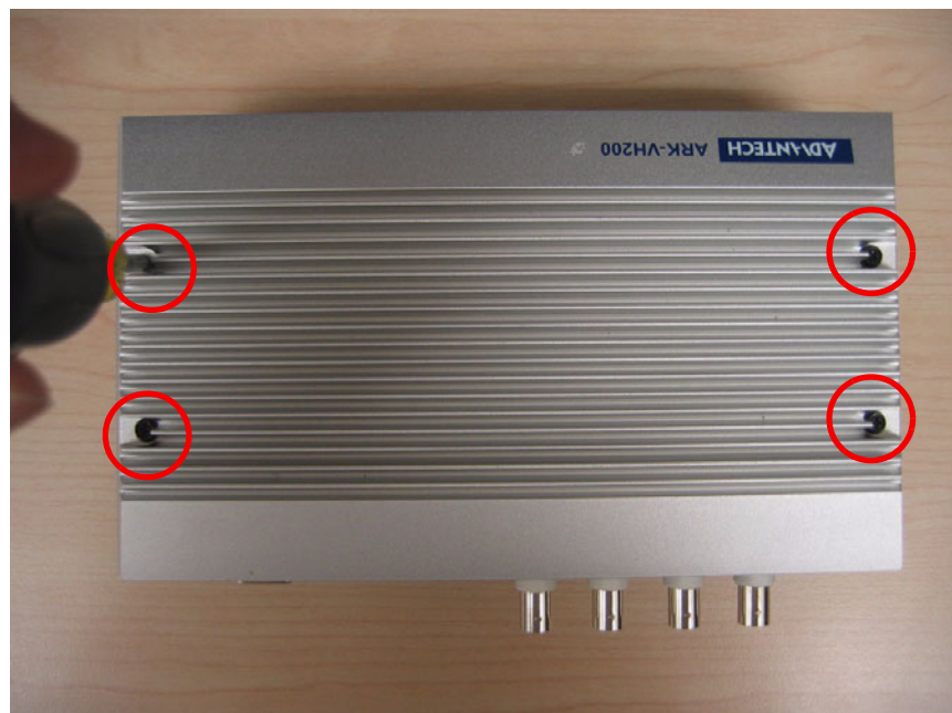
Figure 2.26 Unscrew the top case screws
