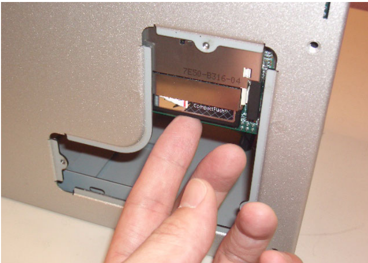
Figure 3.10: Insert the CF card into the CF card slot
