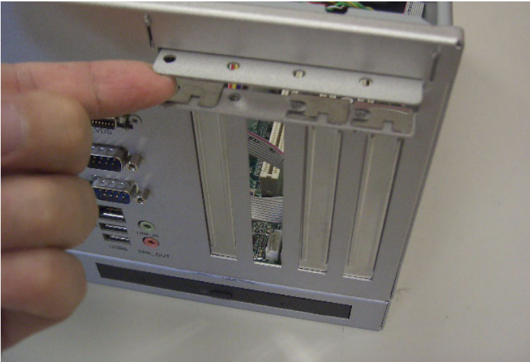
Figure 3.15: Lift the PCI cover bracket and remove the dummy PCI bracket
