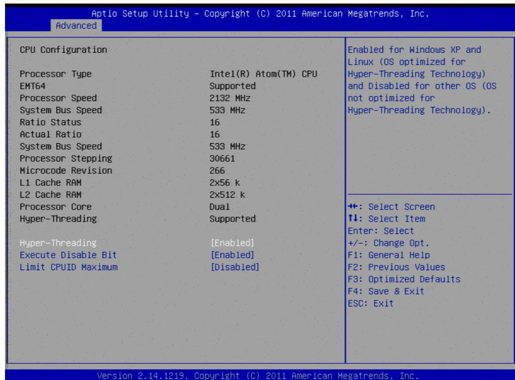
Figure 3.6 CPU Configuration
