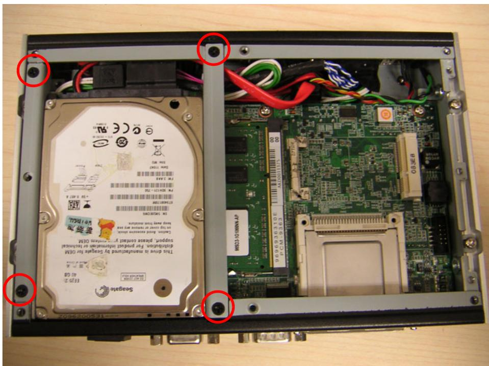
Figure 2.21 Secure HDD
