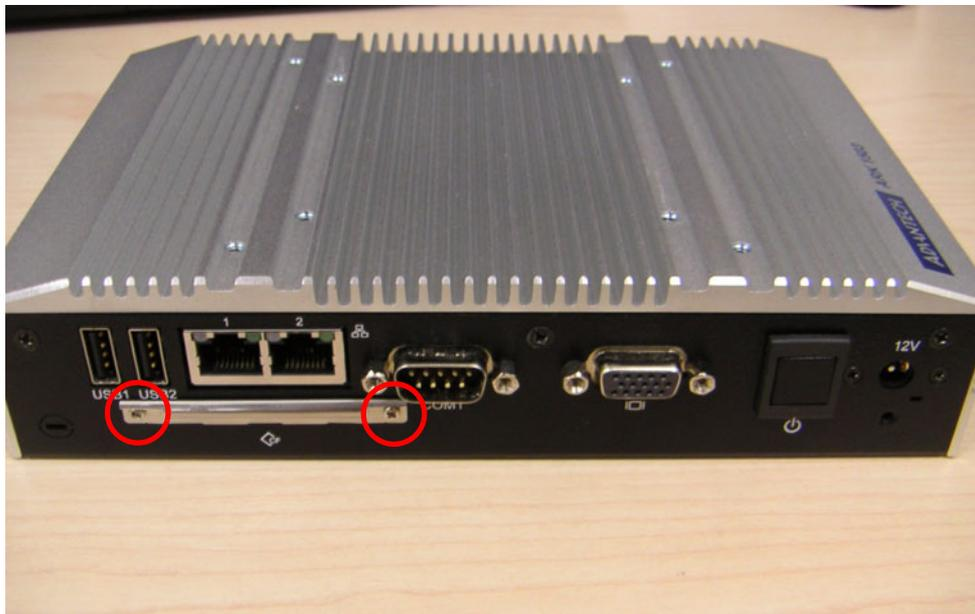
**Figure 2.12 Unscrew the CF door screws**
