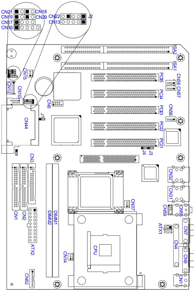
**AIMB-740-B Board Layout: Jumper and Connector Locations**
