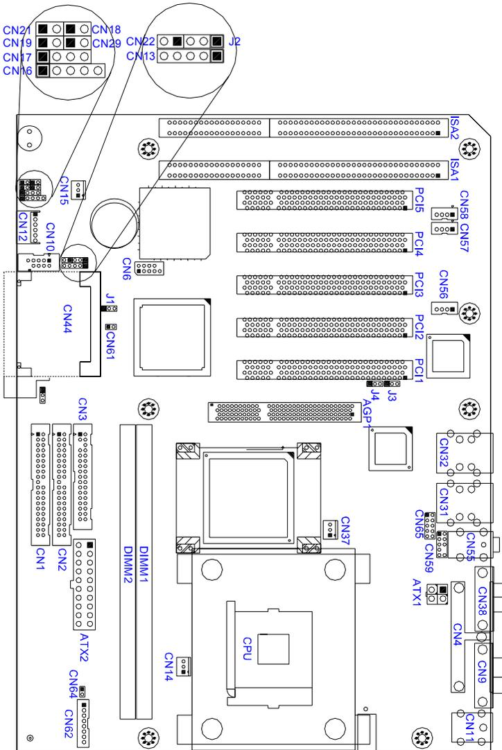
***AIMB-741-B Board Layout: Jumper and Connector Locations***
