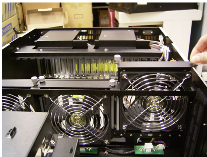
Figure 3.4: Replacing the cooling fan/ 更換冷却风扇 / 更換冷卻風扇
