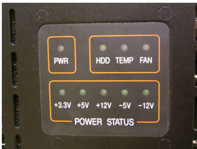
Figure 3.1: LED indicators for system status and power voltage status/ 显示系统和电源电压状态的 LED 指示灯 / 顯示系統和電源電壓狀態的 LED 指示燈
