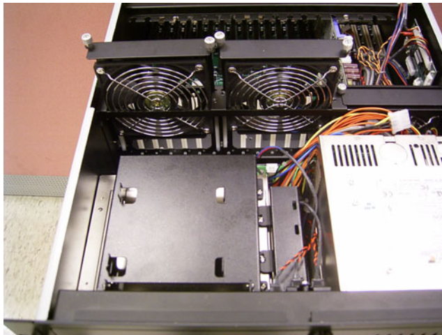
Figure 3.7: First remove the two high-speed cooling fans/ 先移除 2 個高速冷卻風扇 / 先移除 2 個高速冷卻風扇
