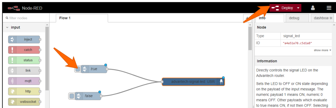
Figure 19: Example 1 – user LED flow
