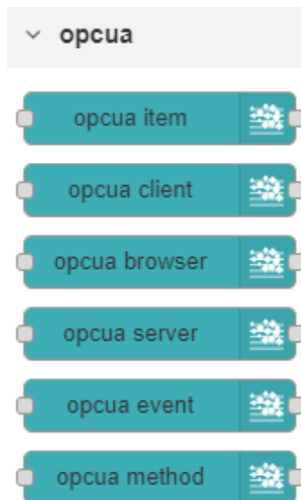
Figure 15: Additional OPC UA node in input list
