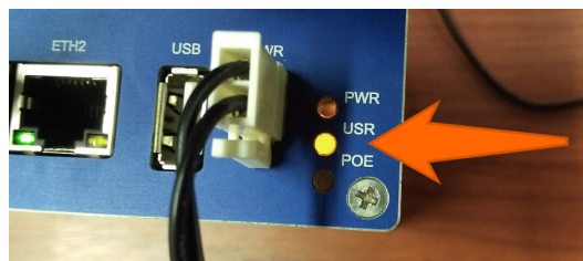
Figure 20: Example 1 – user LED turned on
