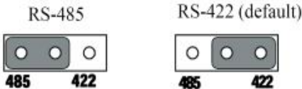
Figure 2.22: RS-422/485 Selection by Jumper Setting
