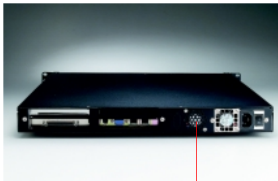
One 10-CFM cooling fan is on rear-end
