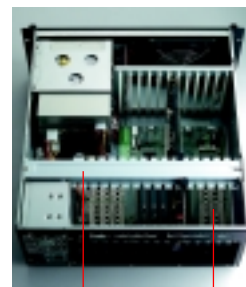
Hold-down clamp Max. 14-slot backplane
