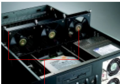
Three 114-CFM hot-swap cooling fans
