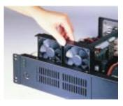
Simply remove two hand screws for easy fan replacement.
