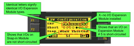
Figure 13. Information Mode: Hardware Configuration
