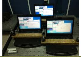
Random Vibration Test: X axis (Battery)
