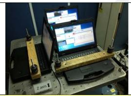
Random Vibration Test: Z axis (Adapter)
