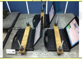
Random Vibration Test: Y axis (Adapter)
