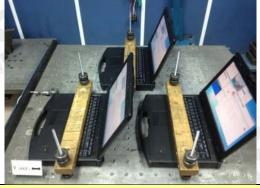
Random Vibration Test: Y axis (Battery)
