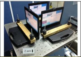
Random Vibration Test: Z axis (Battery)
