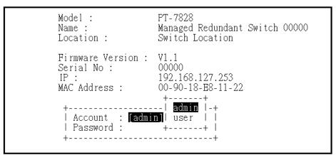
7. The **Main Menu** of the PT-7828's serial console should appear. (In PComm Terminal Emulator, you can adjust the font by selecting **Font...** in the **Edit** menu.)
