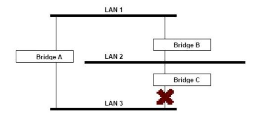
STP will determine which path between each bridged segment is most efficient, and then assign a specific reference point on the network. When the most efficient path has been identified, the other paths are blocked. In the above 3 figures, STP first determined that the path through Bridge C was the most efficient, and as a result, blocked the path through Bridge B. After the failure of Bridge C, STP re-evaluated the situation and opened the path through Bridge B.
