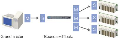
Clock: Determines the time base for the system Boundary Clock: Slave to the grandmaster clock and master to its slave
