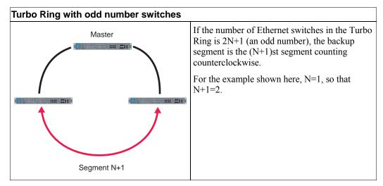
Determining the Redundant Path for Turbo Ring V2
