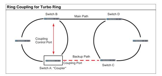
To configure the ring coupling for a **Turbo Ring**, select two PT series Ethernet switches (e.g., Switch A and B in the above figure) in the ring, and another two PT series Ethernet switches in the adjacent ring (e.g., Switch C and D).
