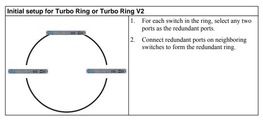
The user does not need to manually assign the master with Turbo Ring or Turbo Ring V2. If no switch is assigned as the master, the protocol automatically selects one of the switches to be the master. The master is only used to identify which segment in the redundant ring acts as the backup path. In the following subsections, we explain how the redundant path is selected for rings configured for Turbo Ring and Turbo Ring V2.
