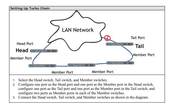
The path connecting to the Head port is the main path, and the path connecting to the Tail port is the back up path of the Turbo Chain. Under normal conditions, packets are transmitted through the Head Port to the LAN Network. If any Turbo Chain path is disconnected, the Tail Port will be activated to continue packet transmission.
