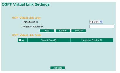
All areas in an OSPF autonomous system must be physically connected to the backbone area (Area 0.0.0.0). However, this is impossible in some cases. For those cases, users can create a virtual link to connect to the backbone through a non-backbone area and also use virtual links to connect two parts of a partitioned backbone through a non-backbone area.
