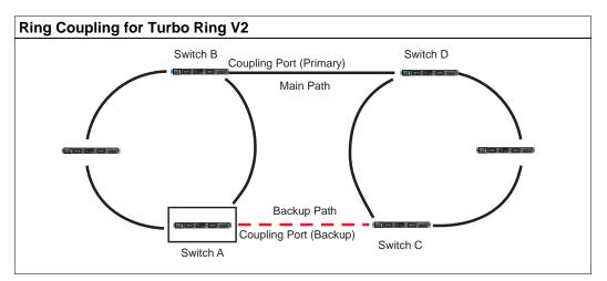
Note that the ring coupling settings for a **Turbo Ring V2** are different from a **Turbo Ring**. For Turbo Ring V2, ring coupling is enabled by configuring the **Coupling Port (Primary)** on Switch B and the **Coupling Port (Backup)** on Switch A only. You do not need to set up a coupling control port, so **Turbo Ring V2** does not require a coupling control line.
