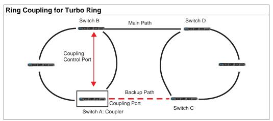
To configure the ring coupling for a **Turbo Ring**, select two IKS series Ethernet switches (e.g., Switch A and B in the above figure) in the ring, and another two IKS series Ethernet switches in the adjacent ring (e.g., Switch C and D).
