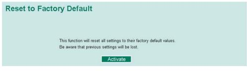
This function provides users with a quick way of restoring the IKS-6726's configuration to factory defaults. This function is available in the serial, Telnet, and web consoles.
