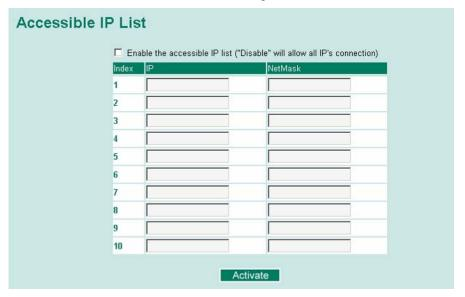
You may add or remove IP addresses to limit access to the IKS-6726. When the accessible IP list is enabled, only addresses on the list will be allowed access to the IKS-6726. Each IP address and netmask entry can be tailored for different situations:
