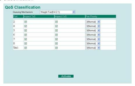
The EDS supports inspection of layer 3 TOS and/or layer 2 CoS tag information to determine how to classify traffic packets.
