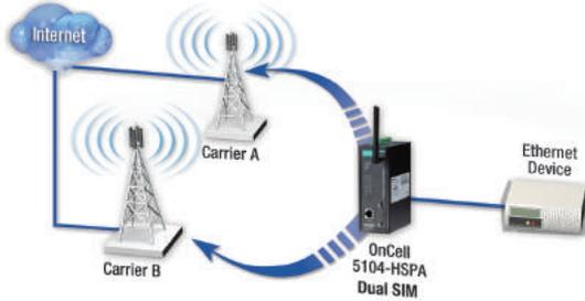
Dual-WAN routing backup service provides the ability to set up primary and secondary WAN connections. For example, setting Ethernet WAN as the primary WAN route means that the router will primarily communicate with remote sites via the Ethernet WAN. If the path is somehow blocked, the router will automatically switch to the cellular WAN as its outgoing route, and vice versa.
