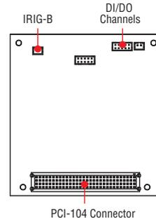
**DA-IRIGB-4DIO-PCI104-EMC4 Hardware Specifications**
