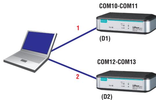
If both UPorts are unplugged from the computer, and UPort® D2 has been plugged back in, the computer will assign COM10 and COM11 to the UPort's serial ports. When UPort® D1 is plugged back in, COM numbers COM12 and COM13 will be assigned the UPort's serial ports.
