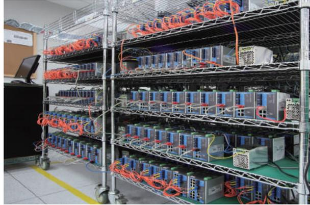
Real-world testing of Turbo Chain with 250 EDS switches
