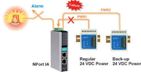
which Ethernet link or power input has failed, or which serial signal has changed. An e-mail warning can also be issued when an exception is detected. These functions are valuable tools that enable maintenance engineers to react promptly to emergency situations.
