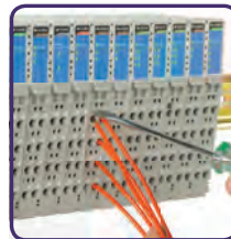
Spring Type Terminal Block
