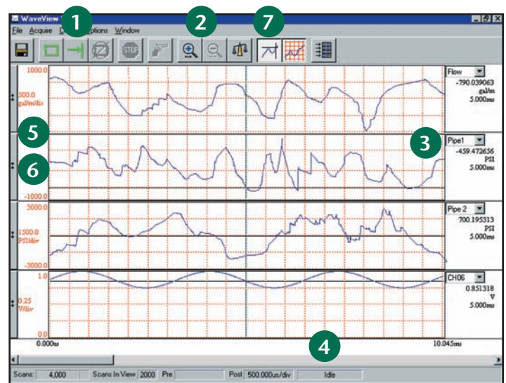
Scope Mode allows you to display any eight of the WaveBooks' channels
