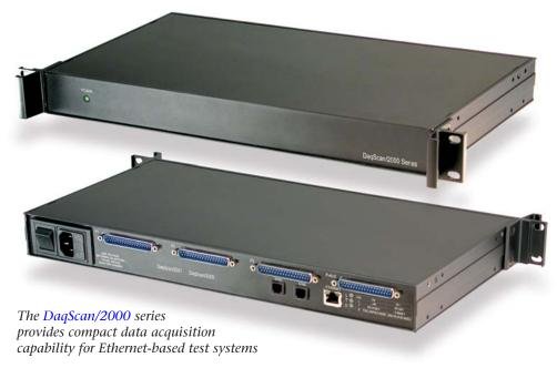
front or the rear of the enclosure. Multiple DaqScan models can be combined in the same system and synchronized using a simple SYNC connection between units. All I/O is accessed via male DB37 connectors located on the rear of the unit, making cabling easy from the DaqScan to your device-under-test.
