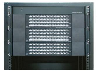
The 168 TC channel system consists of one DaqScan/2005 plus three DBK90 modules with rack-mount kits
