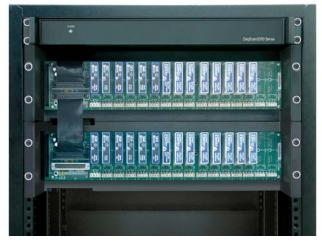
The 32-channel isolated system includes a DaqScan/2005 plus two DBK207/CJC boards. The system is capable of scanning all channels at 5 µsec per channel, and provides 500V isolation for all inputs.
