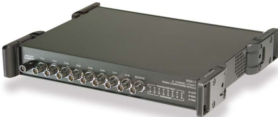
The WBK18 provides a full set of features for making dynamic signal measurements
