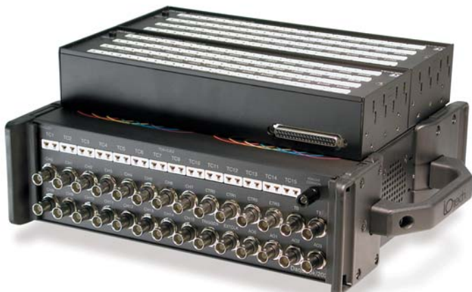
Two DBK90s (112 TC channels) mounted on a DaqBook/2020
