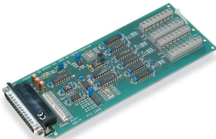
The 8-channel DBK9 RTD card accommodates 3- and 4-wire RTDs
