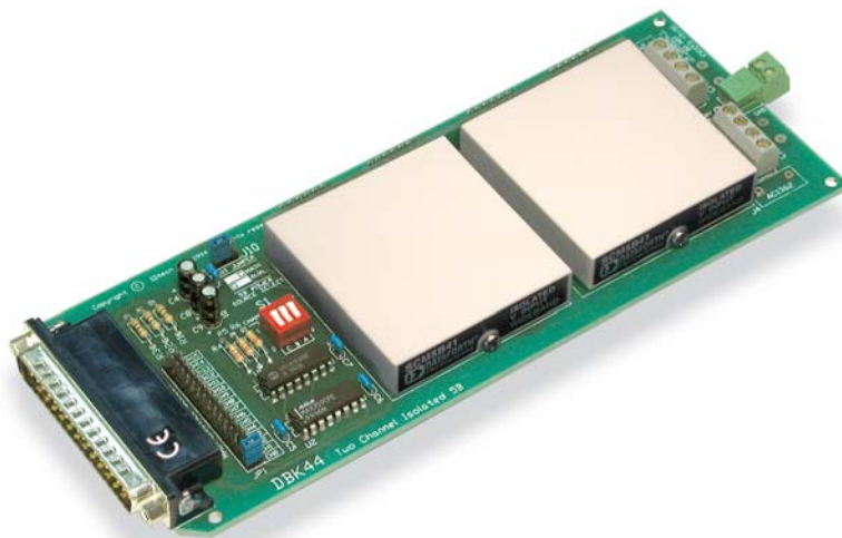
The DBK44 accepts two 5B isolated input signal conditioning modules of any type
