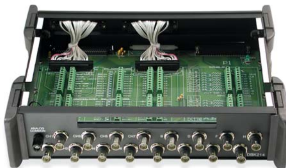
DBK214 shown with cover removed, providing access to all screw terminals
