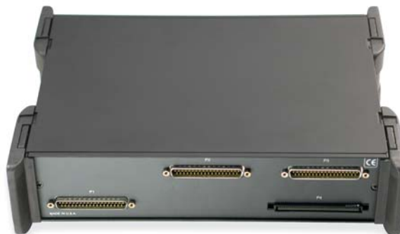
Rear view of DBK214 showing all connections to the A/D host
