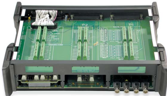
DBK213 shown with cover removed, providing access to all screw terminals
