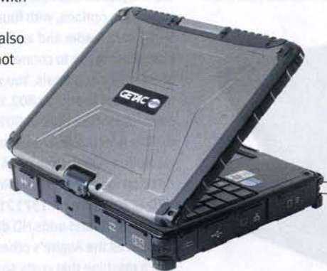
Getac has labelled each of the many rubber flaps with a simple icon to help locate ports.
