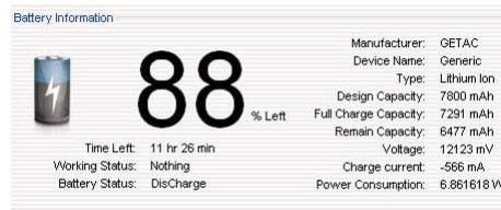
The result was pretty amazing. In continuous operation, the B300 consumed only about 10.5 watts. That is barely more than the ten watts we saw on the Getac E100 tablet with its miserly Intel A110 chip, a testimony to Getac's circuitry and Intel's power management on the
