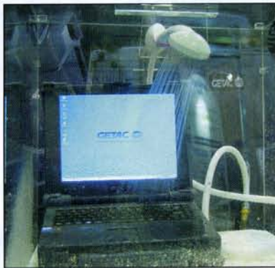
Getac's 'ultra rugged' A790 computer: it has sealed ports and connectors and a removable, shock-mounted hard drive
