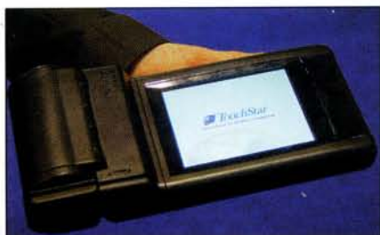
For point-of-sale use, including van sales, the Kestrel computer, with built-in printer. It will also have a chip-and-pin slot for cards
