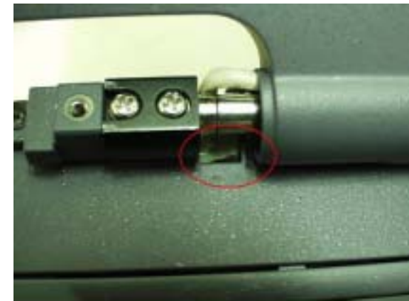
Close bug 8: Rain shower test fail because C part some glue is not add very well
