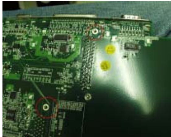
Close Bug 6: Some screw nut at I/O and PCMCIA board will loosed during vibration or shock test
