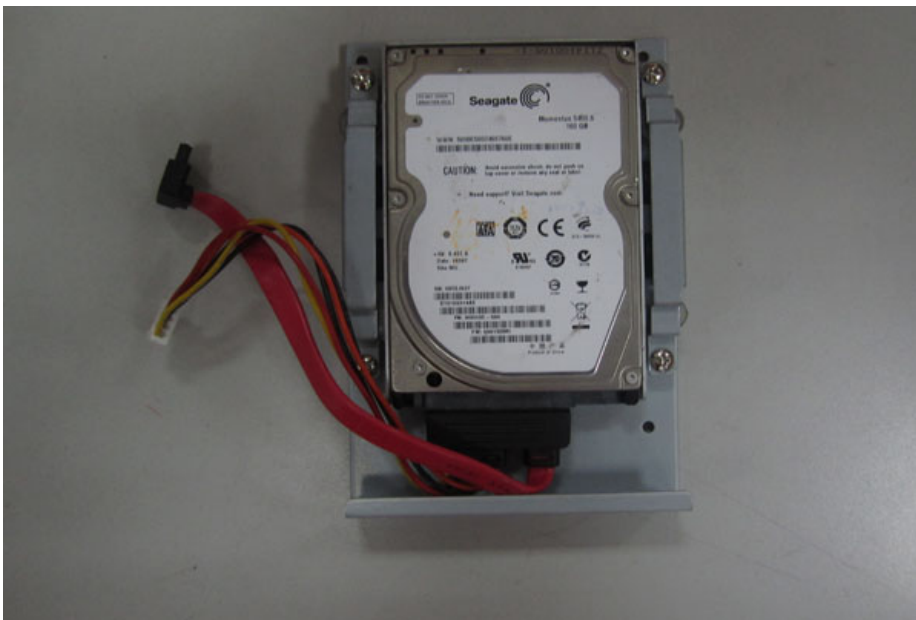
Figure 4.3 Insert SATA HDD Cable on HDD
