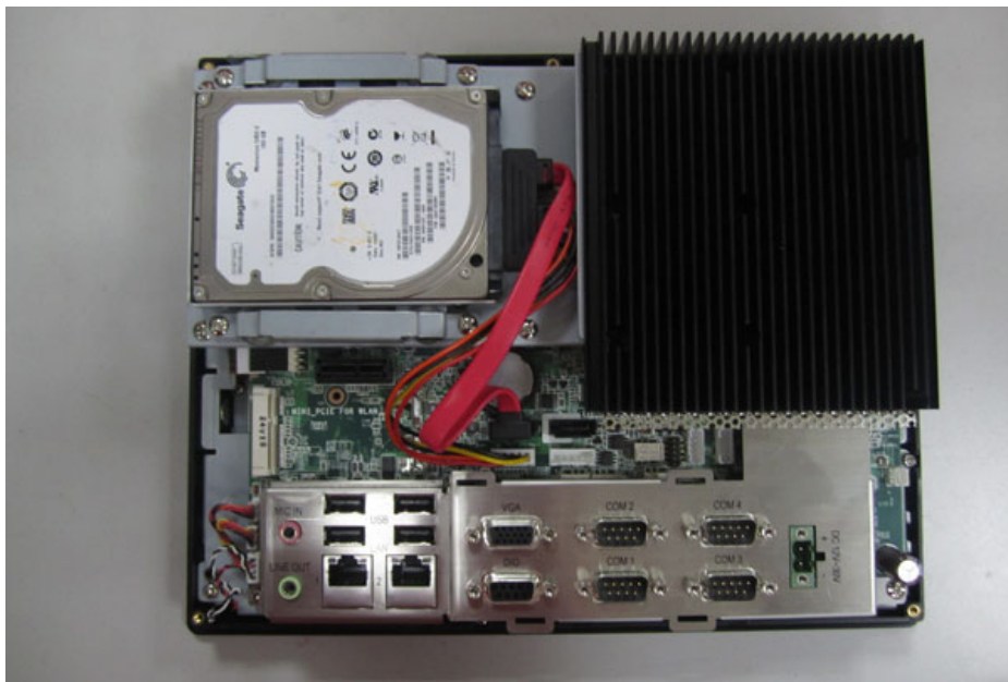
Figure 4.5 Assemble HDD Module on System
