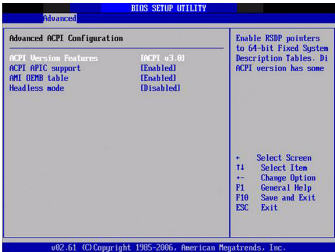
Figure 3.10 Advanced ACPI Configuration
