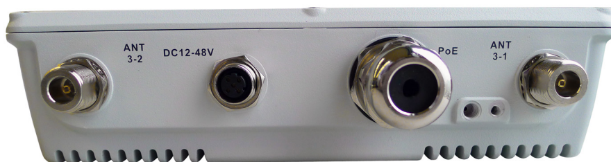
Figure 2.3 Bottom view of data port & power port of Advantech EKI-6340
