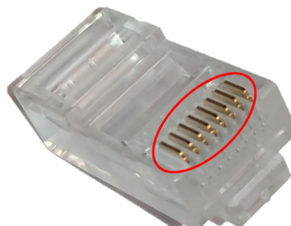
Figure 2.10 Contact plating of the RJ45.
