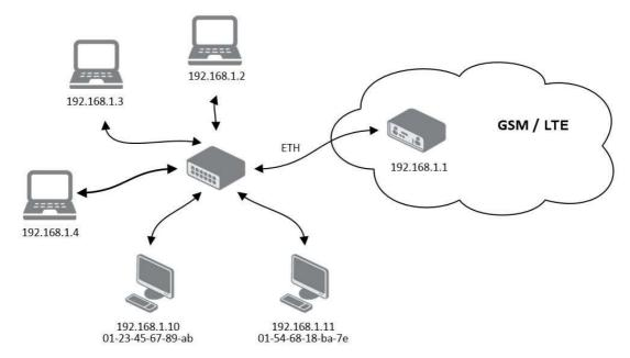
Figure 3.14 IPv4 Dynamic and Static DHCP Network Topology
