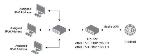
Figure 3.16 IPv6 Dynamic DHCP Server Network Topology
