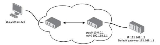
Figure 3.19 Topology for NAT Configuration Example 1
