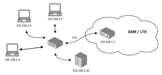
Figure 3.12 IPv4 Dynamic DHCP Network Topology
