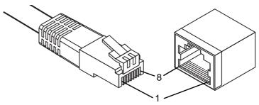
Figure 2.8 Ethernet Plug & Connector Pin Position
