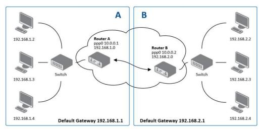
Figure 3.26 Topology of Configuration Example
