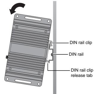
Figure 2.5 Installing the DIN-Rail Mounting Kit
