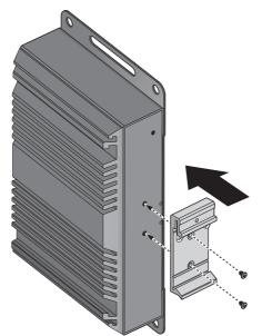
**Figure 2.4 Wall Mount Installation**
