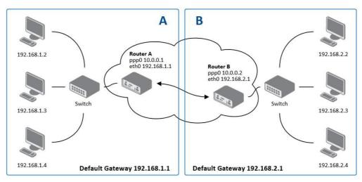
**Figure 3.28 Topology of GRE Tunnel Configuration Example**
