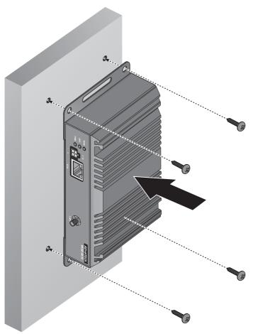
**Figure 2.3 Wall Mount Installation**
