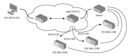
Figure 3.21 Topology for NAT Configuration Example 2
