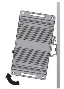
Figure 2.7 Removing the DIN-Rail
