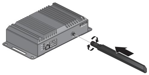
Figure 2.1 Installing the Antenna
