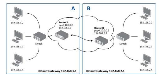
Figure 3.30 Topology of L2TP Tunnel Configuration Example
