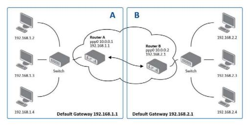
Figure 3.32 Topology of PPTP Tunnel Configuration Example
