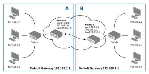
Figure 3.24 Topology of OpenVPN Configuration Example
