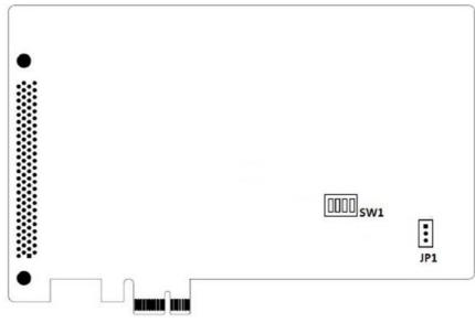
Figure 3.1 Connector and Switch Locations
