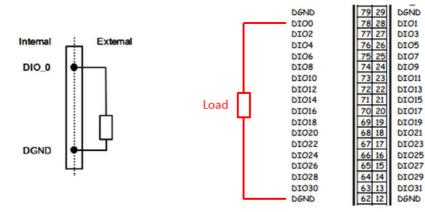
Figure 3.14 Digital Output Channel Connections
