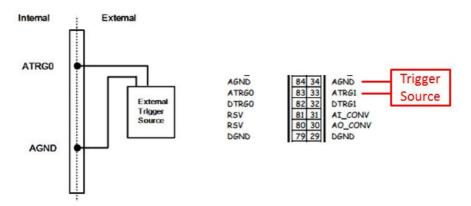
Figure 3.7 External Analog Trigger Source Connection
