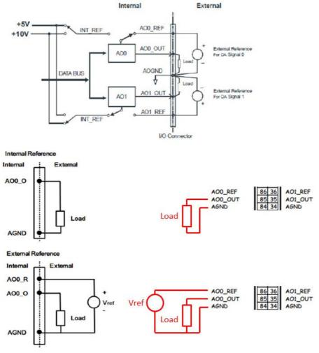
**Figure 3.8 Analog Output Connections**
