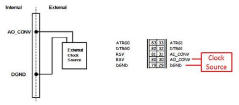
Figure 3.9 External Clock Source Connection
