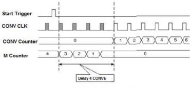
Delay to Start Trigger (M = 4)
