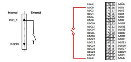
Figure 3.13 Dry Signal Connection of Digital Input
