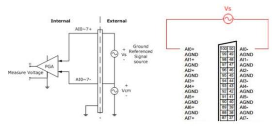
**Figure 3.3 Differential Input Channel Connections**
