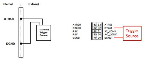
Figure 3.10 External Digital Trigger Source Connection
