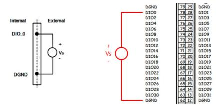
Figure 3.12 Wet Signal Connection of Digital Input
