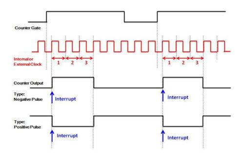
6. **PWM Output:** PCIE-1812 can generate PWM (pulse width modulation) signal which you can configure its logic high time and logic low time as figure below. The available period range for logic high time and logic low time is 100 ns ~ 214 second.
