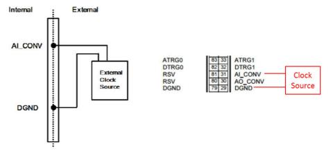
Figure 3.5 External Clock Source Connection
