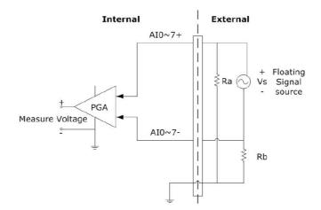
Figure 3.4 Differential Input Channel Connection - Floating Signal Source
