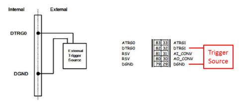
Figure 3.6 External Digital Trigger Source Connection
