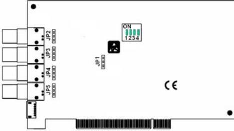
Figure 1: Card Connector, Jumper and Switch Locations
