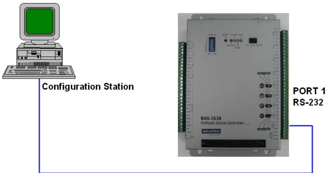
Figure 1.2: Communication with Configuration Station
