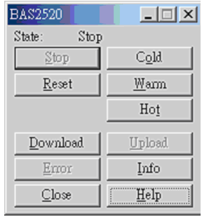
Figure 4.66: Reset PLC CPU via Project Control Dialog
