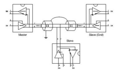
**Figure A.2 Termination Resistor Locations**
