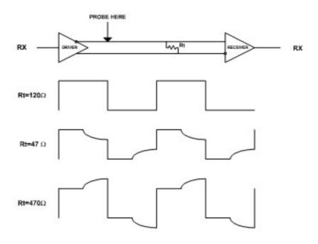
Figure A.1 Signal Distortion
