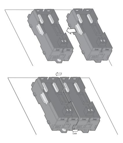
Step 5: Mount that APAX-5002 backplane to the wall (panel) using two standard M4 or #8 panhead screws.
