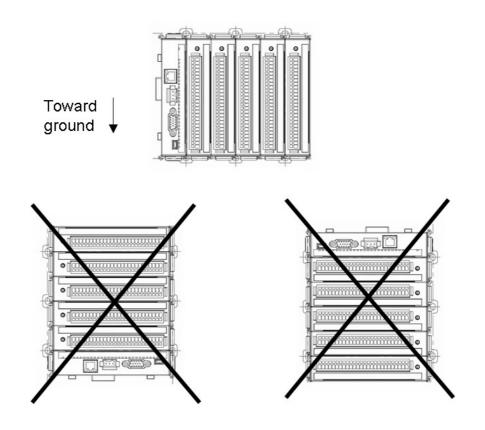
We suggest remaining enough clearance space from enclosure walls and adjacent equipment. No closer than 50 mm (2 in.) apart on all sides, as shown below. This provides ventilation and makes assembly easier.
