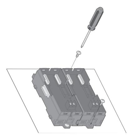
Step 6: Repeat Step 4 ~ Step 5 until all necessary APAX-5002 backplane are screwed on the wall (panel).
