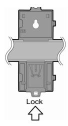
Step 6: Insert the APAX-5620 module and all necessary APAX-5000 I/O modules to the backplanes. (Similar to Step 2, Step 4 and Step 8 in section 3.1.1)
