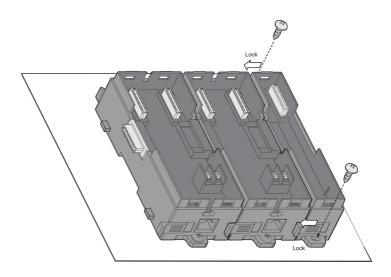
Step 7: Insert APAX-5620 and all necessary APAX-5000 I/O modules to the backplanes. (Similar to Step 2, Step 4 and Step 8 in section 3.1.1)
