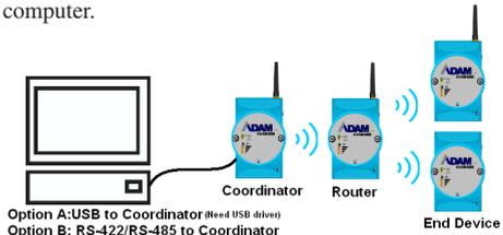
1. Move the right side mode switch of module to Initial Mode for module setup. (Factory default setting is in Normal Mode) Connect type B end of the USB cable to the ADAM-2520Z and the other end to host PC. For RS-422/485 interface user, please connect TX+/-, RX+/- (RS-422) or D+/D- (RS-485) from terminal block to host PC communication port.
