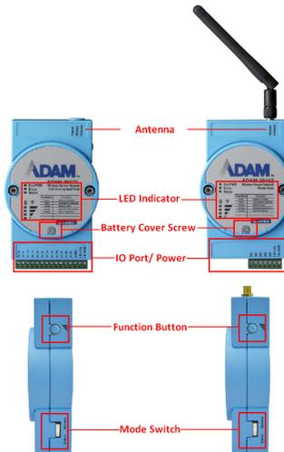
**Normal Mode:** Modules with the same PAN ID & RF channel which will perform self-association to form a Personal Area Network, Router and I/O End Device will send data to Coordinator automatically after power up.
