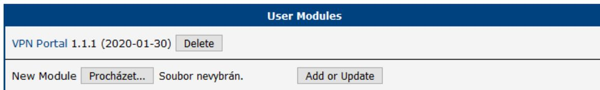
Figure 5: User module *VPN Portal* after upload to the router
