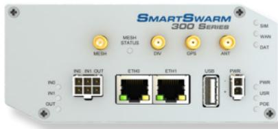
Connect a 2.4GHz antenna to the connector marked "MESH."
