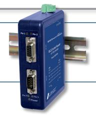
The 2320PDRI is our premium Industrial RS-232 Isolated Repeater. Designed for rugged industrial environments, it is UL listed and certified for use in Class 1 Division 2 locations. Powerful Optical Isolation on both data ports protects your equipment and data from damaging ground loops and surges. Additional isolation on the power supply circuits adds a third degree of protection.
