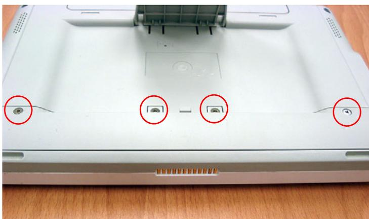
**Figure 2.18** Unfastening the four battery cover screws
