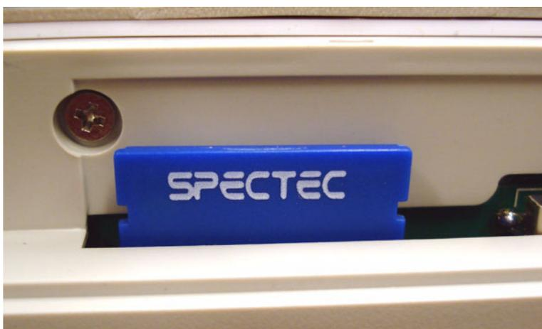
**Figure 2.14** Pushing the WiFi module into the slot
