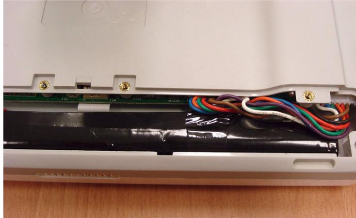
**Figure 2.20 Removing the battery cover**
