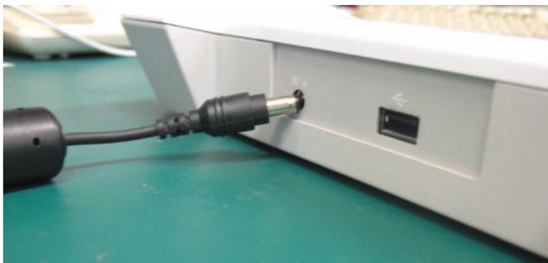
Figure 2.2 Connecting the AC adapter
