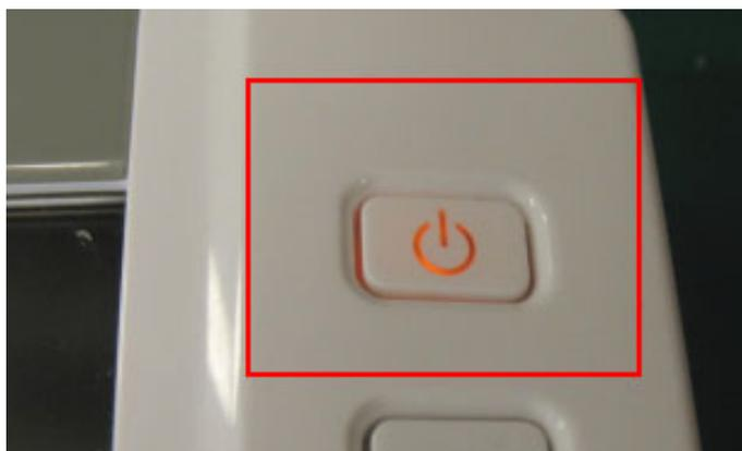
Figure 2.8 Standby mode button orange illumination
