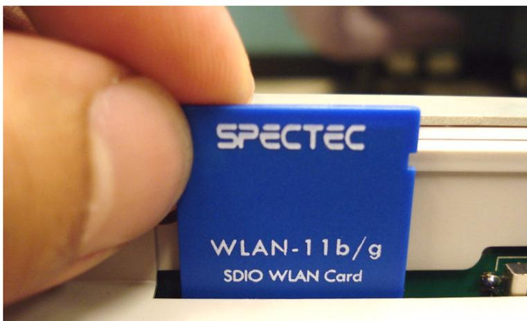
**Figure 2.13** Inserting the WiFi module
