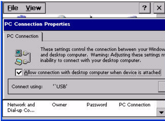
Figure 4.25: PC Connection Properties
