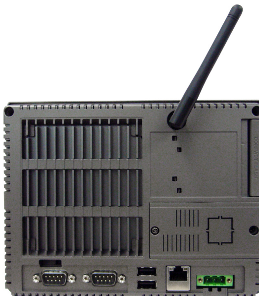
Figure 1.1 TPC-671H - I/O Port Arrangement
