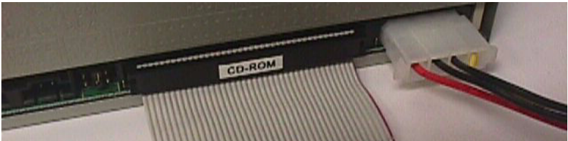
Figure C.7: Plug Power Line into CD-ROM Drive
