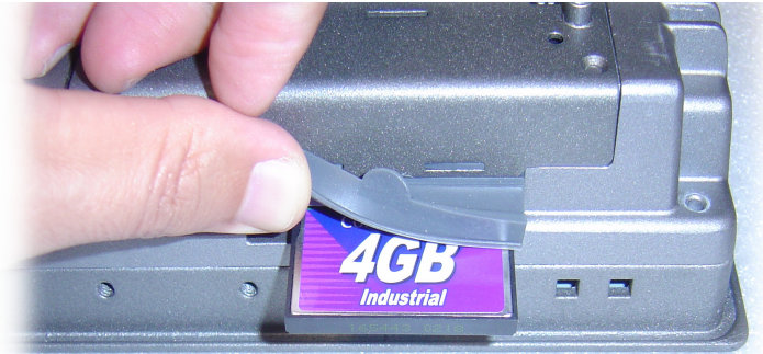
Figure 2.1: Install CompactFlash memory card
